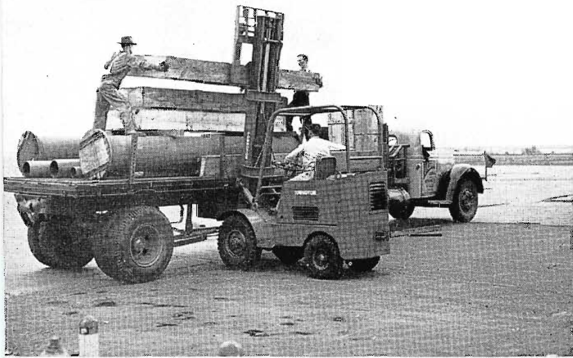
FIG. 7. The three-section Superturnstile and two-section FM Pylon Antennas being transferred from plane to truck at Stapleton Airport, Denver.
