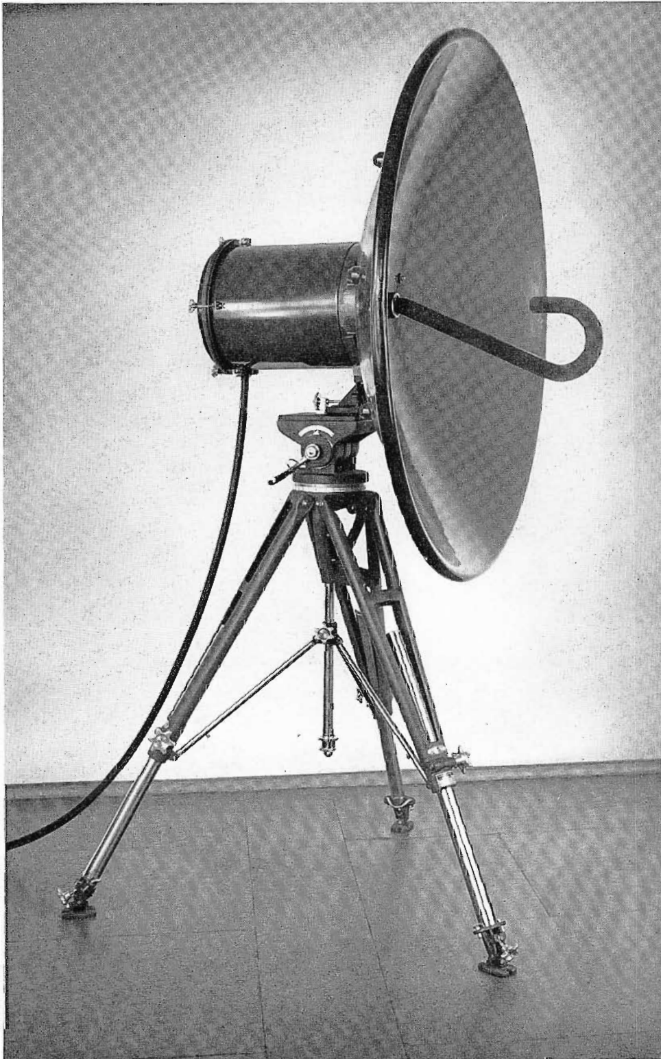
FIG. 1 (at left). Standard RCA TTR transmitter showing feed line for normal (horizontal) polarization. Note in this photo that the RCA relay transmitter is mounted on a new all-metal, lightweight tripod suitable for field use.
