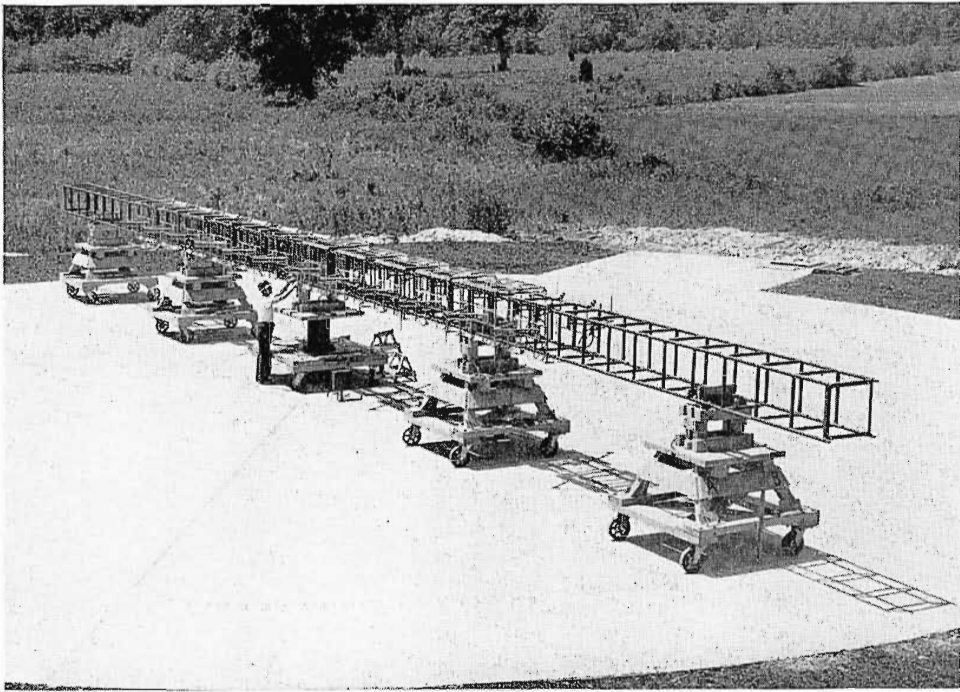
FIG. 13. Supergain and Superturnstile Antennas are tested on this specially built turntable. Antennas up to a length of 140 feet can be mounted, and rotated to determine their radiation characteristics. Transmitting site is located approximately 2400 feet across an open level field.
